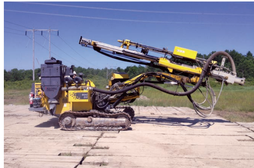
An Atlas Copco D3. In the early 2000s, the AC tethered remote control D3 replaced the 642 and the D7 and began to replace MD&B's workhorse 748.
