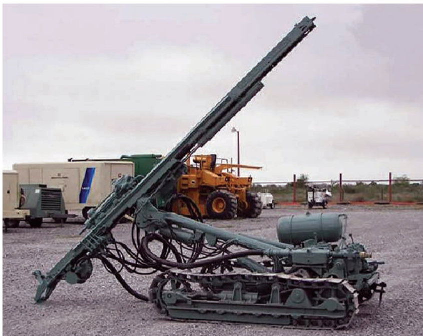
The Gardner Denver Air Track Drill in the 1970s.
