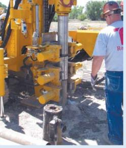
mer, AMS Inc. and Sonic Sampling & Supply demonstrated the capabilities of their Compact Roto-Sonic 17-C in American Falls, Idaho. Drillers from all over the United States and Canada watched the unit quickly and easily core through solid rock, collect core samples and create a borehole for a geothermal loop in-
