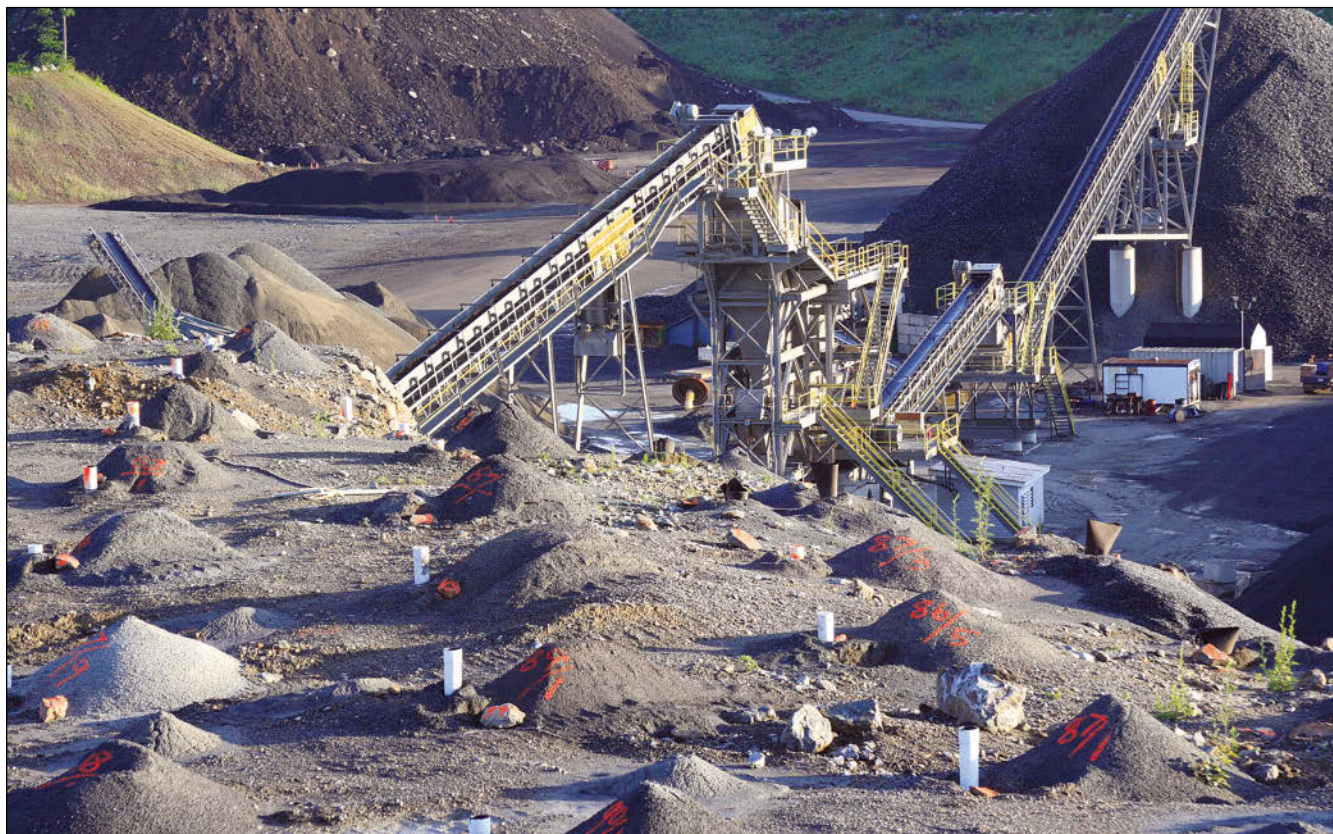
Photo courtesy of Maine Drilling & Blasting MD&B introduced electronic detonator technology in Brox Industries' Dracut, Maine, quarry to provide advanced control for a blast that used 70,000 lbs. (31,751 kg) of explosives in an area in which $20 million in immovable quarry structures existed within a 225-ft. (69 m) radius of the blast. Post blast, there were just under 130,000 tons (117,934 t) on the ground, almost 100 percent crushable, with no damage to any structures and no complaints from area residents.
