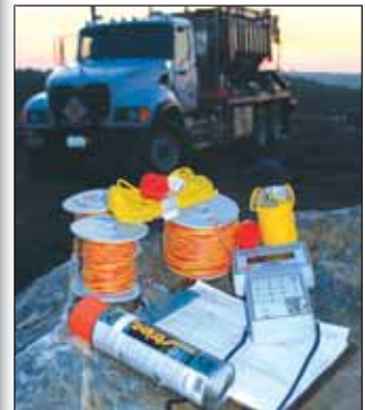
Bulk truck and electronic equipment at sunrise start to load the shot.
