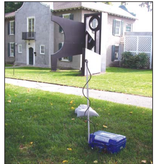
Seismograph setup at The Hyde Collection, Glens Falls, NY.
